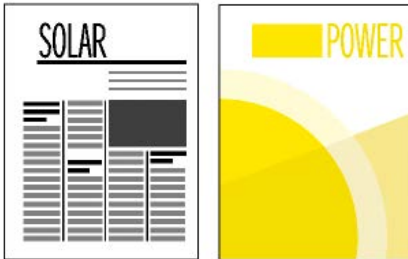
A. Composite image B. Black separation C. Spot color separation
